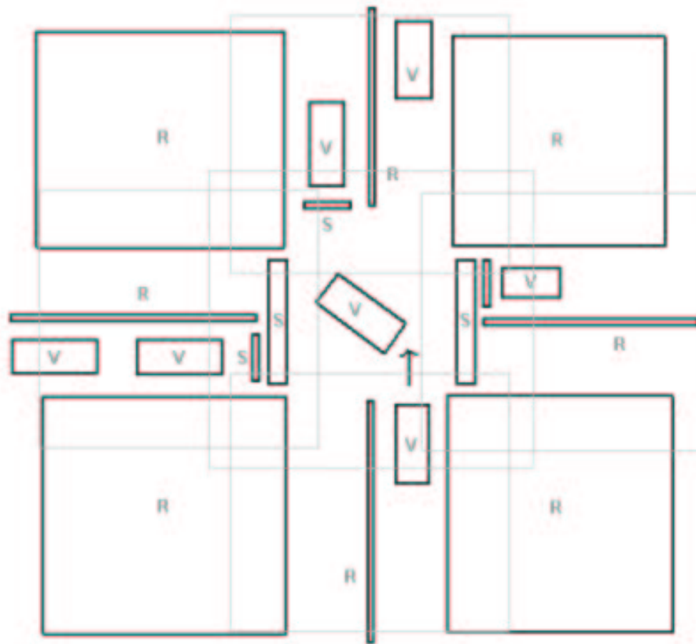
Figure 3: Intersection features modeled as geometric entities. R, V, and S are geometric representation of road features, vehicles and signals respectively. The thin lines show the partition scheme used for computing the occupancy list in the two-step collision prediction algorithm.
