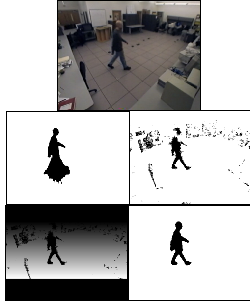
Figure 6. Foreground process (left to right): Source image, background subtraction image containing shadow, chromaticity subtraction image, weighted chromaticity subtraction image, and composite mask with shadow removed.
